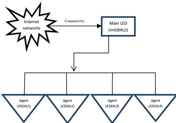
**Figure 1.** Architecture of Li-Fi technology
