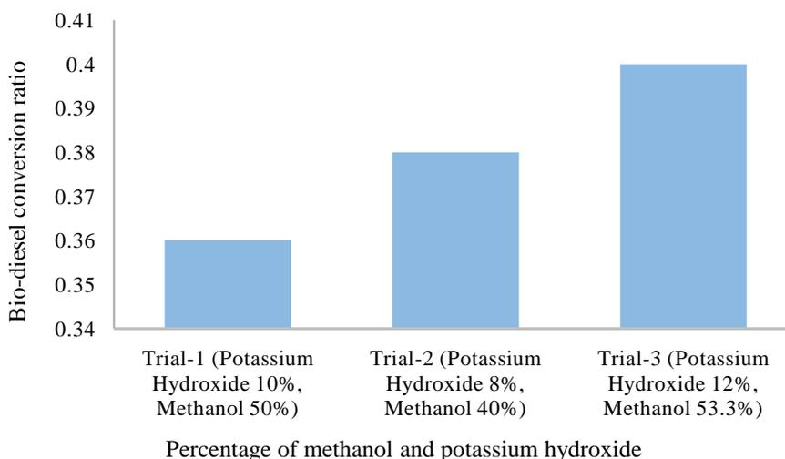
**Figure 3.** Bio-diesel yield conversion ratio with methanol and potassium hydroxide percentage
