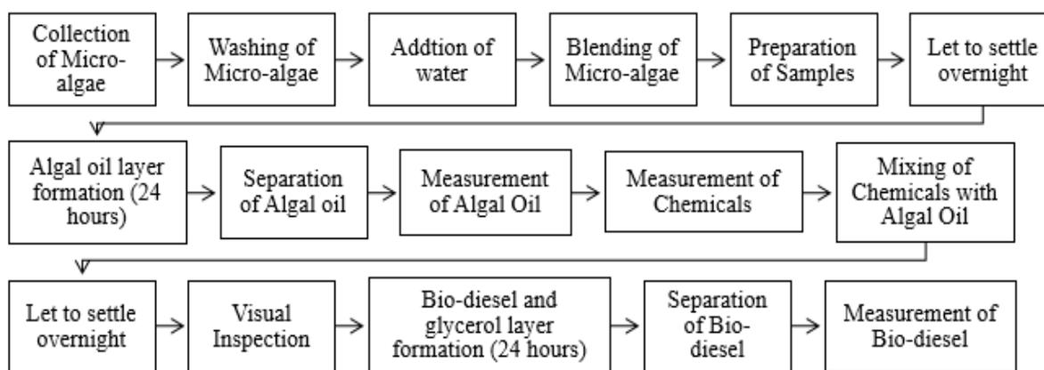
**Figure 1.** Layout of bio-diesel production
