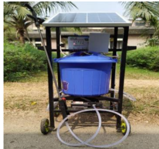
Figure 2. A photographic view of solar-powered sprayer
