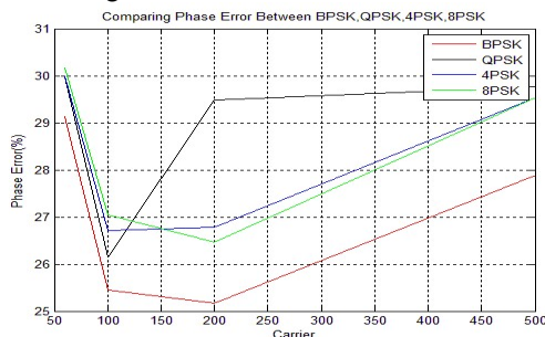
Figure 3. Phase Error for different subcarrier in case of BPSK, QPSK, 4PSK and 8PSK
