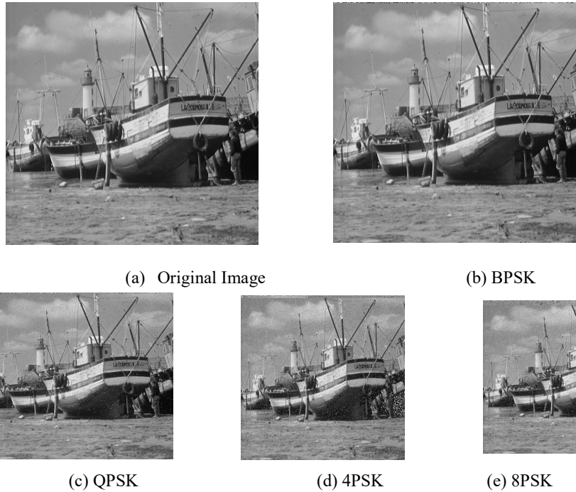
Figure 8. Image Quality of received Image verses transmitted image for SNR=10
